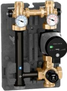
Thermostatic adjustable temperature mixing unit with insulation. Grundfos UPS 15-58 three speed pump. Grundfos Alpha 25-55U pump. Temperature gauges. Shut-off ball valves. Compatible with 5599 Hydrolink series. Male union connections (select top and bottom fitting sets below). Max working pressure: 145 psi. Adjustable range: 80–125°F. Power supply: 115 V 50/60 Hz.
