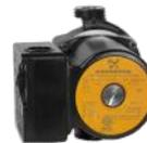
Replacement single speed 120 V, 1" male union thread. Flow 36 feet head / 8 gpm. Agency approval: cULus. (install in-line with NA122 union fittings on page 94)
