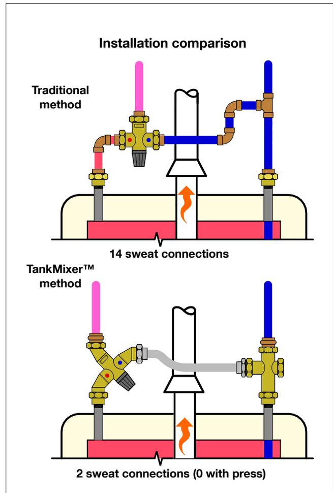
Meets requirements of NSF/ANSI 372-2011. Certified to ASSE 1017, CSA B125.3, UPC, IPC, Low Lead Laws and listed by ICC-ES for use in accordance with the U.S. and Canadian plumbing codes.
