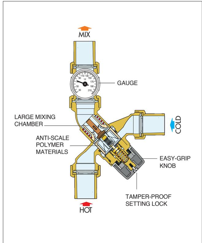
Meets requirements of NSF/ANSI 372-2011. Complies with ASSE 1017, CSA B125.3, UPC, IPC, Low Lead Laws and listed by ICC-ES for use in accordance with the U.S. and Canadian plumbing codes.
