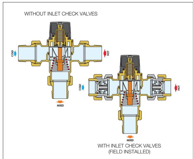
THERMOSTATIC MIXING VALVES FOR PLUMBING AND HYDRONICS
