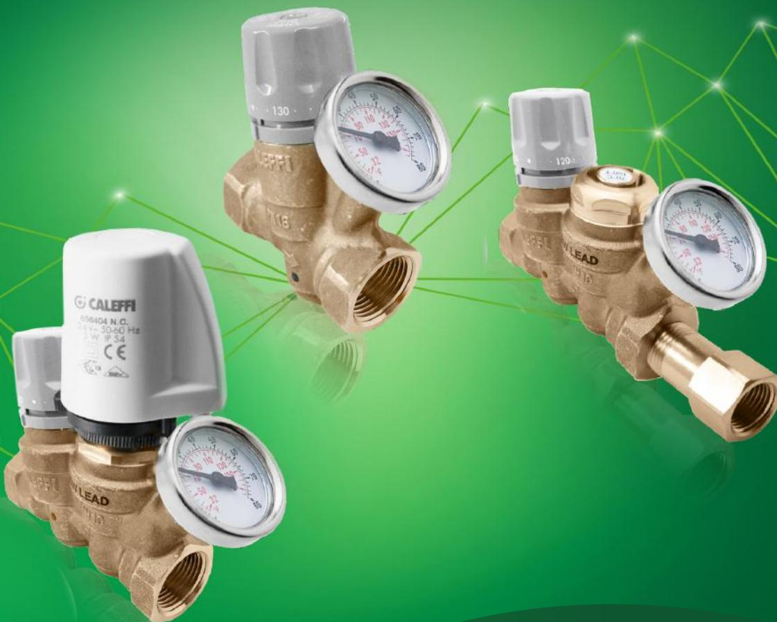
The **ThermoSetter™** thermal balancing valve maintains precise temperature in recirculation return piping using state-of-the-art modulating control. **Setup is simple** and safe with an easy-to-read, lockable temperature adjustment dial. The integral drywell is versatile, suitable for a local slide-in temperature gauge or remote sensor bulb. Models with bypass cartridges are available for projects that are designed for **thermal disinfection to control Legionella bacteria. CALEFFI GUARANTEED.**
