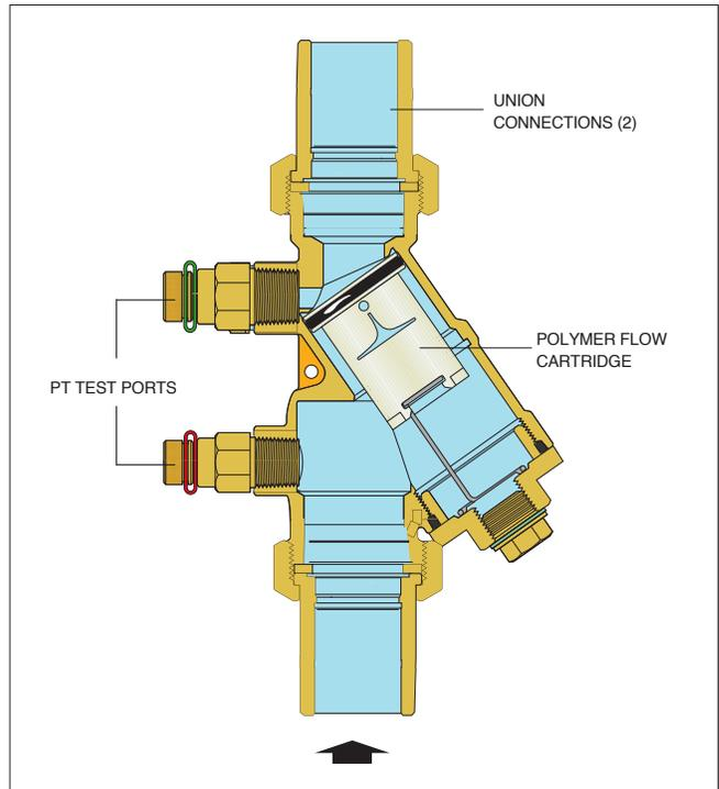
**STATIC BALANCING VALVES, FIXED ORIFICE, FOR PLUMBING AND HYDRONICS**
