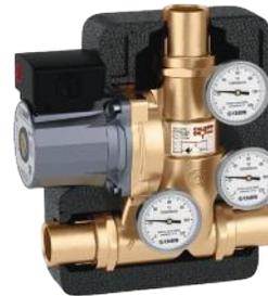
ThermoBloc™ boiler protection recirculation and distribution unit. Suitable fluids: water, up to 50% glycol solutions. Max. working pressure: 150 psi. Working temperature range: 40—210°F. Maximum pumping capacity: 10 gpm. Temperature gauge scale: 30—250°F. Thermostatic sensor: 130°F & 140°F Tset standard selections, see below. 115°F, 160°F Tset optional models\*. Sensor cartridge accuracy: ±4°F. By-pass from boiler complete closing temperature: Tset +18°F (ex. 130°+18°=148°F). \* Consult factory
