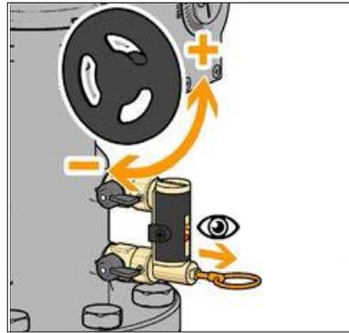
The 132 series balancing valve accurately sets the flow rate of heating and cooling transfer fluid. The flow meter is housed in a bypass circuit on the valve body and can be shut off during normal operation. The flow meter permits fast and easy circuit balancing without added differential pressure gauges and reference charts.
