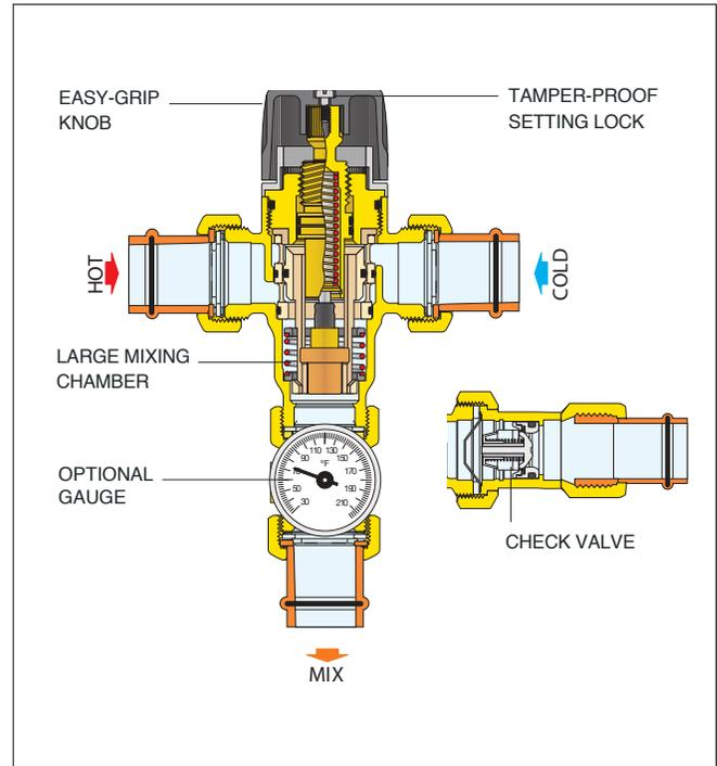
**HIGH FLOW THERMOSTATIC MIXING VALVES FOR PLUMBING AND HYDRONICS**
