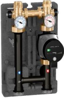
Injection pump mixing unit with insulation. Grundfos UPS 15-58 three speed pump. Grundfos Alpha 25-55U pump. Temperature gauges. Shut-off ball valves. Compatible with 5599 Hydrolink series. Male union connections (select top and bottom fitting sets below). Max working pressure: 145 psi. Max. working temperature: 212°F. Power supply: 115 V 50/60 Hz.
