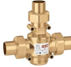
Boiler protection high-flow thermostatic mixing valve. Changeable thermostatic sensor cartridge. Brass body and lower plug. Max. working pressure: 150 psi. Working temperature range: 40—212°F. Thermostatic sensor cartridge: 130°F & 140°F Tset standard selections, see below. 115°F, 160°F Tset optional (field replaceable). Sensor cartridge accuracy: ±4°F. By-pass from boiler complete closing temperature: Tset +18°F (ex. 130°+18°=148°F).
