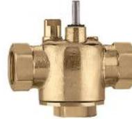
Three-way on/off two position valve. Diverting flow pattern. Brass body. Stainless steel stem. EPDM rubber seals and paddle. Max. working pressure: 300 psi. Max temperature: 240°F.
