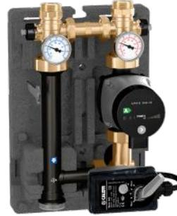
Motorized temperature mixing unit with insulation. Three-point floating 24 VAC actuator for use with separately-sourced outdoor reset controller. Grundfos UPS 15-58 three speed pump. Grundfos Alpha 25-55U pump. Temperature gauges. Shut-off ball valves. Compatible with 5599 Hydrolink series. Male union connections (select top and bottom fitting sets below). Max working pressure: 145 psi. Primary inlet temperature range: 40-212°F. Power supply: 115 V 50/60 Hz. Valve actuator: 24 V AC
