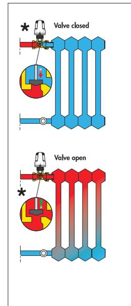
**NPT THERMOSTATIC RADIATOR VALVE BODIES**
