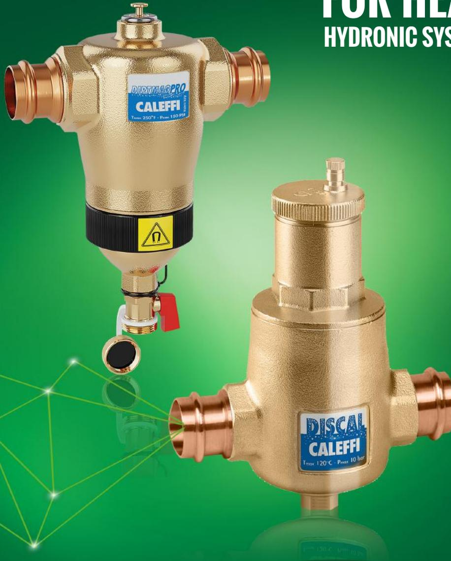
The **DISCAL**® air separator and **DIRTMAG PRO**® dirt separator duo ensures maximum protection and efficiency in hydronic systems. The DISCAL high efficiency air separator features a large, low-flow zone, coalescing element and automatic air vent to minimize corrosion formation. The DIRTMAG's magnetic technology and particle mesh removes both ferrous and non-ferrous debris helping to keep expensive heat exchangers and ECM circulators running smoothly. **CALEFFI GUARANTEED.**
