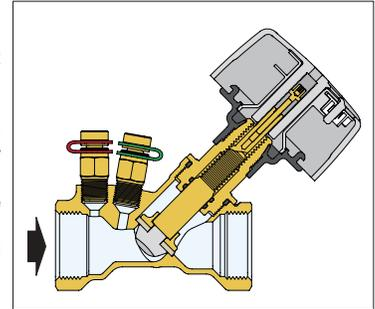
**STATIC BALANCING VALVES, VARIABLE ORIFICE, FOR PLUMBING AND HYDRONICS**
