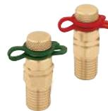
Fast-plug pressure/temperature test ports fits FlowCal™ automatic flow balancing valves and the 120 series Y-strainer. The double-sealing core insures long and trouble free service. Low Lead brass body. Nordel Core. Connections: ¼" NPT male. Cap thread: ⅜"-24 UNF. Working temperature range: 0–275°F. Max. working pressure: 435 psi. Pair (2 ports included).
