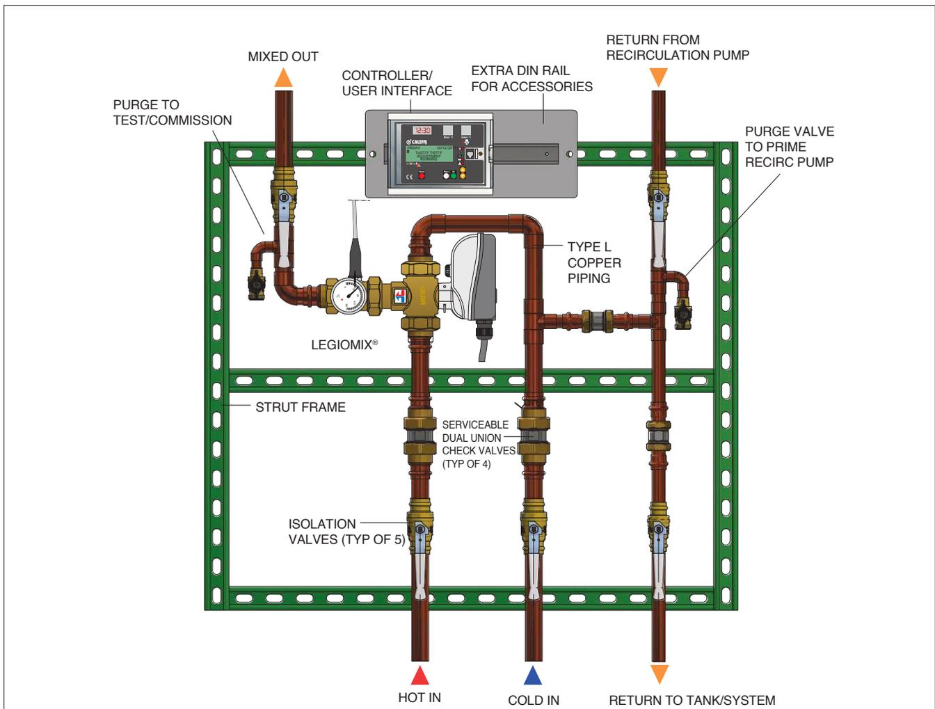
THERMOSTATIC MIXING VALVE KIT FOR DOMESTIC WATER HEATERS
