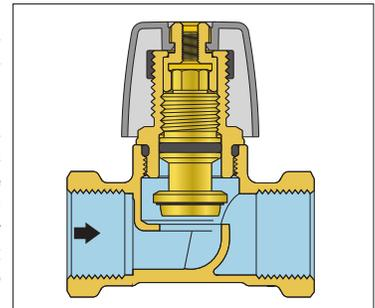
**THERMAL BALANCING VALVES FOR PLUMBING**
