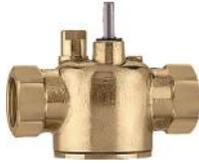
Two-way on/off two position valve. Straight through flow pattern. Brass body. Stainless steel stem. EPDM rubber seals and paddle. Max. working pressure: 300 psi. Max temperature: 240°F.
