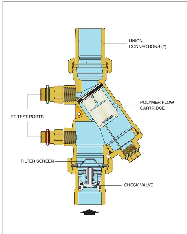
**DYNAMIC BALANCING VALVES FOR PLUMBING AND HYDRONICS**
