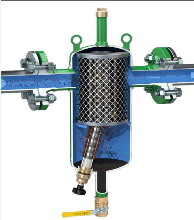
To purge the debris, the flexible magnetic stack is removed from the brass dry-well and, even while the system is still running, the drain valve is opened. Aided by the system pressure, the dirt and magnetite flushes out quickly and effectively. DIRTMAG magnetic dirt separators accomplish 2½ times the ferrous impurities removal performance of standard dirt separators, delivering up to 100% elimination efficiency.
